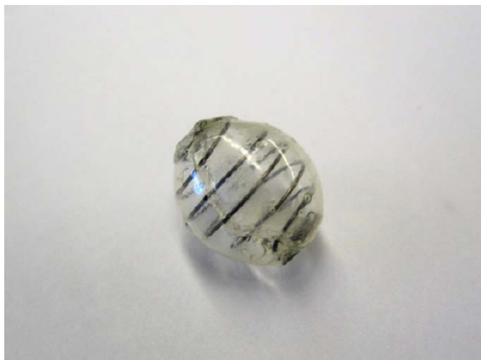
Figure S1. Picture of the coil-in-shell device before implantation.
